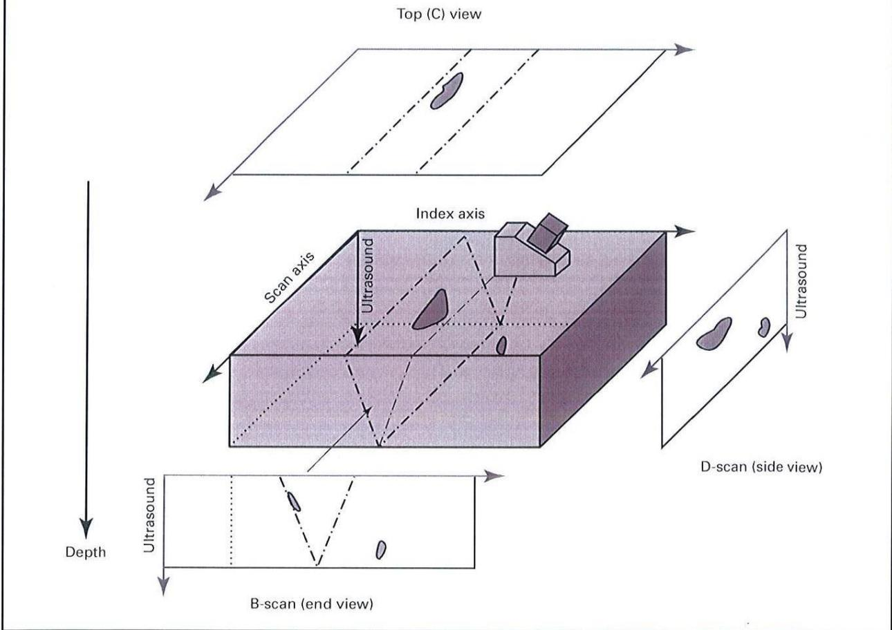
**Figure 4: Volume-corrected B-scan, C-scan and D-scan displays**
